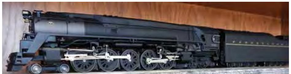
*The PRR's class Q1 comprised a single experimental steam locomotive for freight service, #6130, built in March 1942. A duplex locomotive, it had a wheel arrangement of 4-6-4-4, comprising a four-wheel leading truck, two sets of driving wheels (six followed by four) in a rigid locomotive frame, and a four-wheel trailing truck.*
